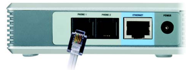
Figure 3-2: Connect the RJ-11 Telephone Cable
